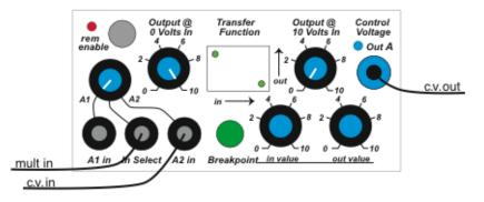
Now add a break point, such that the output stays at a constant 2 volts until the average of two inputs exceeds 8 volts – then the output voltage rapidly goes to 10 volts:
